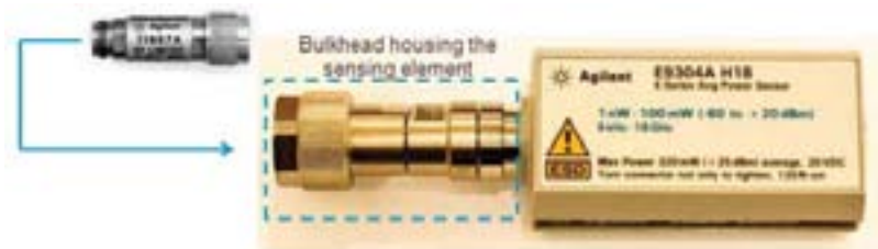
Figure 2. The bulkhead of a power sensor
