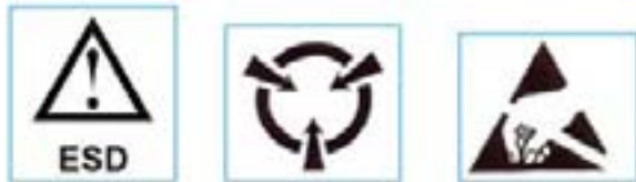
Figure 15. Labels used on power sensors to indicate their sensitivity to ESD
