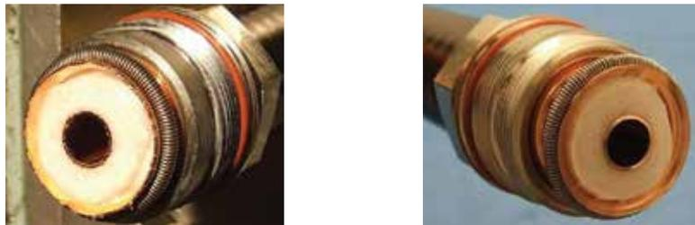
**Figure 4: Cable ends should be clean, square, properly de-burred and free of debris.**
