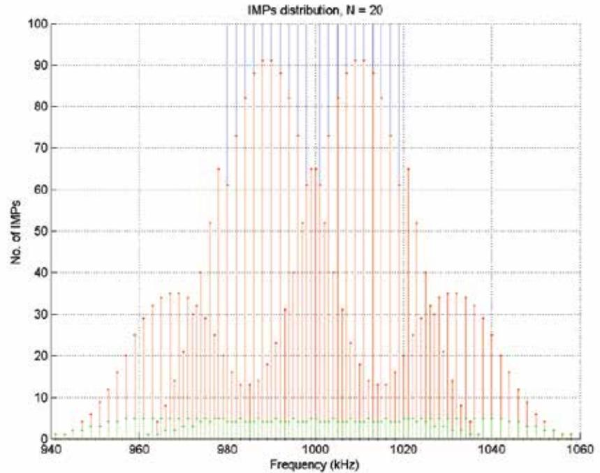
**Figure 2: Multi-tone signal third-order intermodulations indicating the fundamental carriers (blue), dominant IMPs (red) and specific IMPs (green).<sup>10</sup>**
